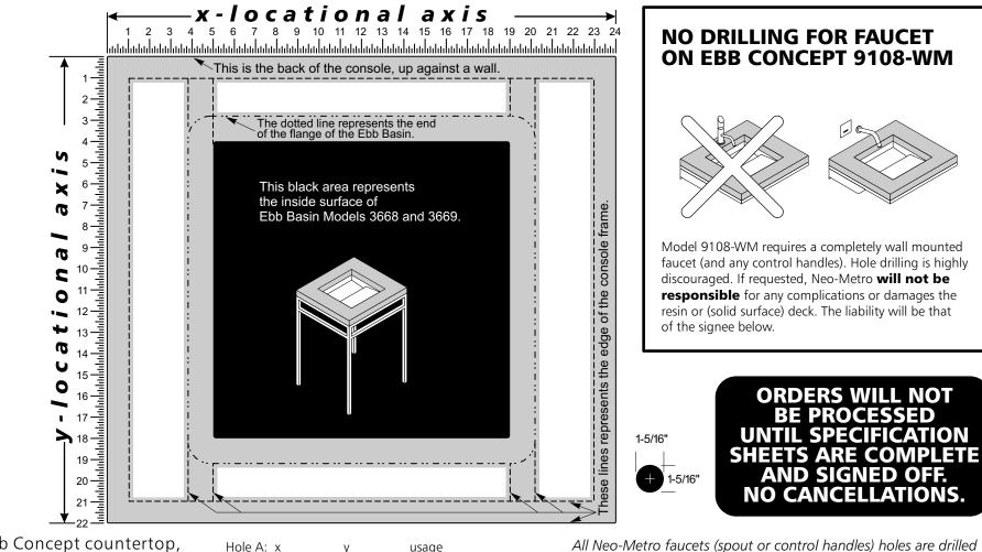
All Neo-Metro faucets (spout or control handles) holes are drilled 1-5/16" (33.3mm) diameter in the resin or solid surface. If the client is going to use another faucet not provided by Neo-Metro, a specification sheet of that faucet must be submitted and signed off in addition to this sheet.
